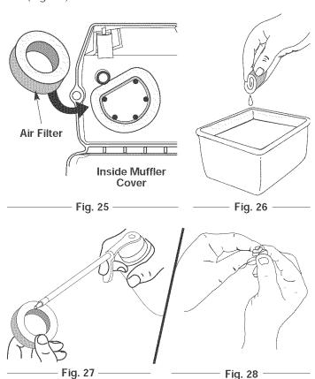
6. Replace the air filter inside the air filter/muffler cover (Fig. 25).
