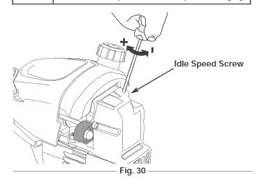
Release the throttle trigger and let the engine idle. If the engine stops, insert a small phillips or flat blade screwdriver into the hole in the air filter/muffler cover (Fig. 30). Turn the idle speed screw in, clockwise, 1/8 of a turn at a time (as needed) until the engine idles smoothly.
