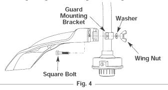
3. Put the washer on the bolt, then screw the wing nut onto the bolt and tighten. Figure 5 shows the installation process from underneath the unit.
