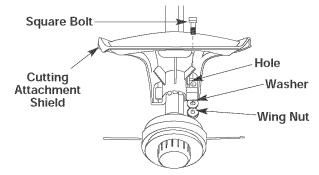
**Cutting Attachment and Shield: Underside View**
