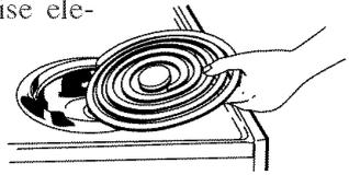
**To replace:** Insert terminals on the element into receptacle. Guide the element into place. Gently press down on the outer edge of the element until it sits level on the drip bowl.
