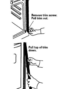
Remove trim screws attaching right and left side trim to oven. Grasp the bottom end of trim and pull away from oven. Slide top end of trim downward to remove trim from oven. Take care not to scratch other surfaces with ends of trim. Set trim and screws aside on protected surface.
