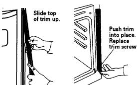
■ Slide top end of each trim upward onto oven side rails. Push each trim into place at bottom of trim. Use screws to attach each trim to oven. Take care not to scratch other surfaces with ends of trim.
