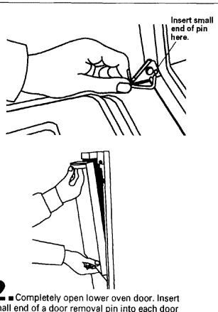
Completely open lower oven door. Insert small end of a door removal pin into each door hinge. Grasp door handle from the bottom and gently close door as far as it will shut. Lift slightly and grasp bottom of door with other hand. Pull door out at bottom to remove. Set door aside on protected surface.
