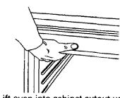
■ Lift oven into cabinet cutout using the oven opening as an area to grip.
