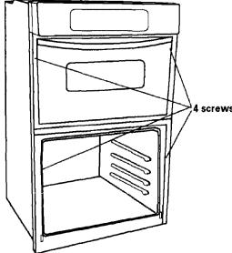
**6** ■ Important: Securely fasten oven to cabinet using the screws provided (two screws for a single oven or four screws for a double oven). Insert the screws through holes in mounting rails. Do Not overtighten screws.
