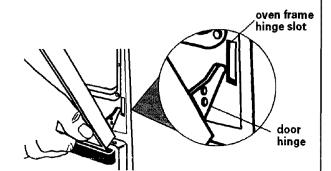
Replace the lower oven door by inserting ends of hinges into hinge slots in oven frame. Push behind each hinge so that hinges are pushed into oven frame as far as they will go. Open door and remove both door removal pins. Close and open door to check that door closes and opens completely. If door does not close or open completely, you have not pushed hinges completely into frame. Repeat door removal step and reinsert door into hinge slots again.
