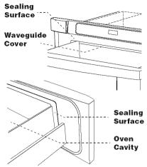
drawer, damaged drawer seals and sealing surfaces, broken or loose drawer guides and dents inside the cavity or on the front side of the drawer. If there is any damage, do not operate the Microwave Drawer and contact your dealer or a SHARP AUTHORIZED SERVICER.
