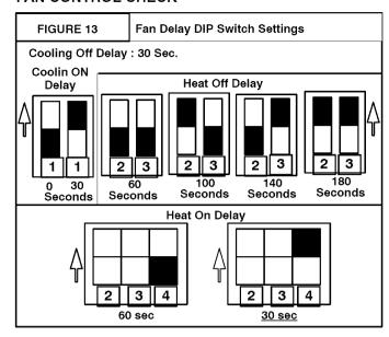
The Fan Control has adjustable settings for the circulating air blower to delay it "ON" and "OFF".
