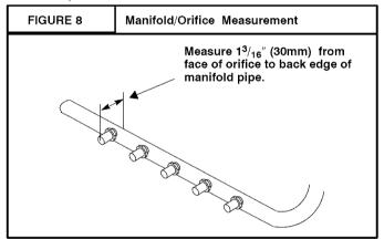
Install the correct orifices. Gauge the size of the orifices with a new twist drill bit of the correct size.
