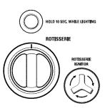
**NOTE:** The location of the rotisserie burner makes it susceptible to strong wind conditions, more so than the protected grill burners. For this reason you should avoid utilizing the rotisserie burner during windy conditions. As an added precaution we've equipped the burner with an automatic safety valve which will not allow gas to flow to the rotisserie burner unless the following conditions are present with the knob on:
