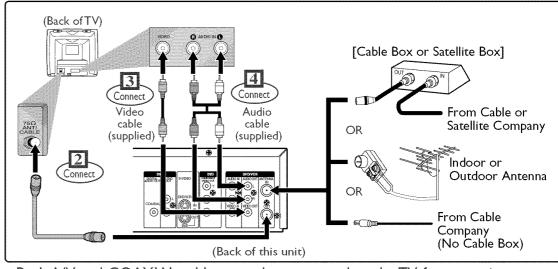
• Both A/V and COAXIAL cables must be connected to the TV for operation.
