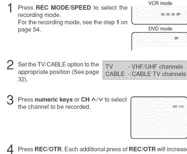
Press REC/OTR. Each additional press of REC/OTR will increase recording time as shown in the chart below, up to a maximum of 6 hours. The OTR and recording time will appear on the screen for about 4 seconds.
