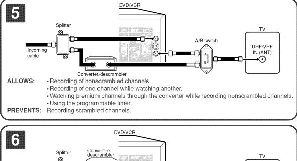
A/B switch UHF/VHF Incoming cable Converter/descrambler ALLOWS: • Recording of all channels through the converter box. • Recording a scrambled or unscrambled channel while watching another (scrambled or unscrambled) channel. • Using the programmable timer to record only the channel selected at the converter box. PREVENTS: Using the DVD/VCR tuner to select channels.
