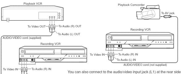
You can also connect to the audio/video input jack (L1) at the rear side of this unit. In addition, each S-Video input jack at the front and rear sides can be used for recording on the disc. (The S-Video input jack cannot be used for recording on the video tape.)
