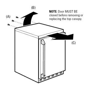
**CAUTION:** Under side edges of the stainless steel canopy top may be sharp. Wear heavy-duty work gloves when moving the top.
