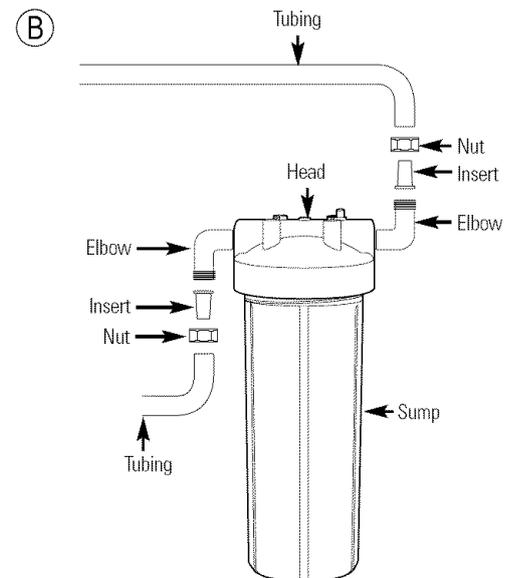
**NOTE:** Avoid installing the unit where the tubing is pulled at a sharp angle. This type of installation may cause the fittings to leak. If using tubing other than what is supplied, be sure it is high quality, exact size and roundness, and has a smooth surface.
