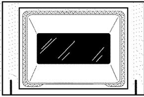
The gasket is designed with a gap at the bottom to allow for proper air circulation. Do not rub or clean the door gasket—it has an extremely low resistance to abrasion.
