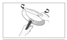
Pans should have flat bottoms that make good contact with the entire surface element. Check for flatness by rotating a ruler across the bottom. There should be no gaps between the pan and ruler.
