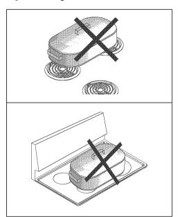
**Woks** with flat bottoms suitable for use on your cooktop are available in most cookshop or hardware stores. Round-bottomed woks (with a support ring that does not extend beyond the heating element) may also be used. The metal ring was designed to support the wok safely when it is filled with large amounts of liquids (soup making) or fat (frying).
