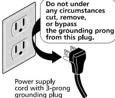
Power supply cord with 3-prong grounding plug
