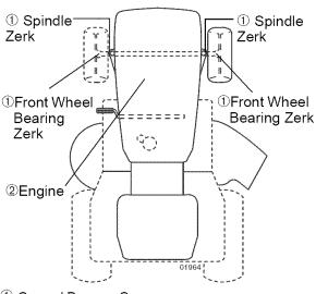
① General Purpose Grease 2 REFER TO Maintenance "ENGINE" SECTION
