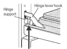
Lock engaged for door removal Figure 1
