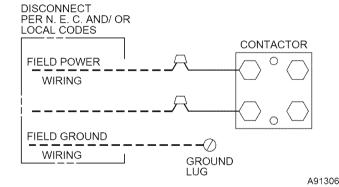
Fig. 11—Line Power Connections
