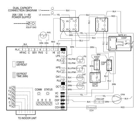
→ Fig. 17—Wiring Diagram—024, 036, 048
