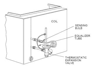
Fig. 5—TXV Installed
