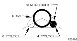
Fig. 7—Positioning of Sensing Bulb
