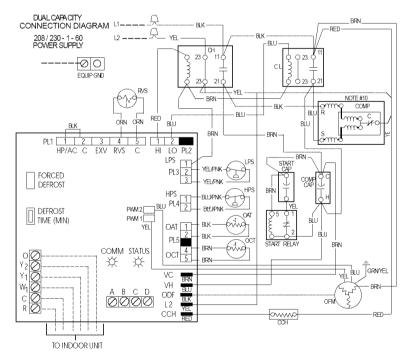
→ Fig. 18—Wiring Diagram—037
