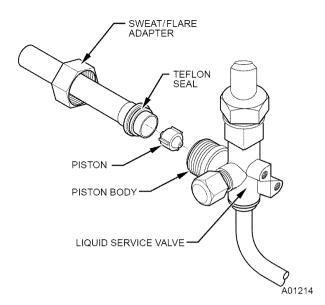
Fig. 8—Liquid Service Valve with Sweat Adapter Tube
