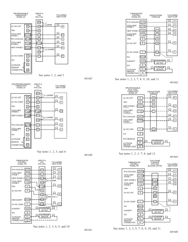
Fig. 12—Typical 24V Circuit Connections
