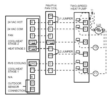
→ Fig. 13—Typical Solenoid Valve Wiring
