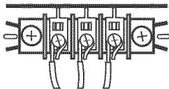
1. Loosen or remove center terminal block screw.
