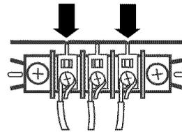
4. Tighten strain relief screws.
