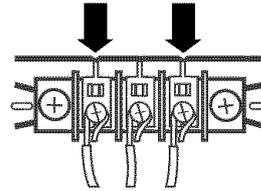
6. Tighten strain relief screws.
