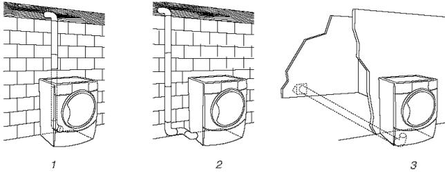
1. Standard rear offset exhaust installation
