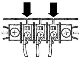
4. Tighten strain relief screws.
