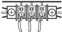
1. Remove center terminal block screw.
