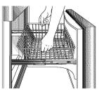
5. Remove Phillips screw from each side of rail system (select models).
