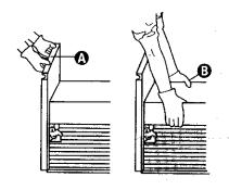
**3.** Place two corner posts from carton on floor near compactor. Open compactor drawer and remove any shipping materials or other items shipped in drawer. Do Not remove compactor bag (if installed). Grasp
