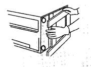
4 Place the other two corner posts on the floor to the side of compactor. Grasp sides of compactor cabinet and put compactor on its side on top of corner posts. Remove shipping base from bottom of compactor.
