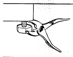
6 Use pliers to lower leveling legs away from cabinet. Adjust legs so there will be 1/8" (3 mm) to 1/4" (6.4 mm) space between top of compactor and top of cabinet opening. Stand compactor upright.
