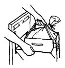
**5** Lift bag by bag caddy handles. Remove trash bag from compactor and dispose properly.
