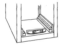
Place level inside on floor of cabinet. Check that compactor is level from front to back and side to side. Adjust leveling legs until compactor is level.
