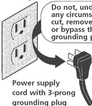
Power supply cord with 3-prong grounding plug
