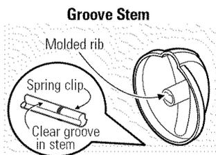
The knob stem has a groove in each side. The groove on one side has a spring clip. The other groove is clear (see illustration). Check the inside of the knob and find the molded rib.
