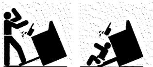
If your range is removed for cleaning, servicing or any reason, be sure the anti-tip device is reengaged properly when the range is replaced. Failure to take this precaution could result in tipping of the range and cause injury.
