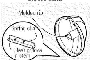
The knob stem has a groove in each side. The groove on one side has a spring clip. The other groove is clear (see illustration). Check the inside of the knob and find the molded rib.
