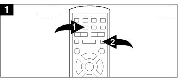
To Repeat play a track/file, simply select the track/file as described on the previous page, then press the REPEAT button **①** twice "REP 1" will appear on the TV screen and the unit will repeat the selected track/file continuously until the STOP button **②** is pressed.
