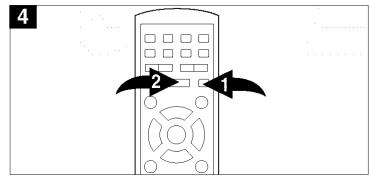
To stop playback, press the Stop ( $\blacksquare$ ) button ①; "PRESS PLAY KEY TO CONTINUE" will appear on the TV screen. Because the unit will remember where you stopped, simply press the Play ( $\triangleright$ ) button ② to resume playback where you left off (resuming playback).
