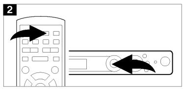
Press the OPEN/CLOSE button to open the disc tray, "OPEN" will appear on the screen and in the display. Insert a disc will the label side facing up on the disc tray.
