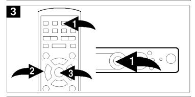
Press the OPEN/CLOSE button ① to close the disc tray. "LOAD" will appear on the screen and in the display. After loading, the menu screen of the DVD should appear. Use the Navigation ( $\blacktriangleleft$ ,  $\blacktriangleright$ ,  $\blacktriangle$ ,  $\blacktriangledown$ ) buttons ② to select the desired option and the ENTER button ③ to select it.
