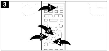
Press the OPEN/CLOSE button ① to close the disc tray. "LOAD" will appear on the screen and the display. After loading, playback will start immediately. Press the NAVIGATION ( $\triangle$ ,  $\heartsuit$ ) button ② to select the desired track. Press the ENTER button ③ to start the playback.
