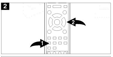
Press the 3D button once ① and the sound options will appear on the screen. Press the  $\blacktriangleright$  button ② to select BAND to view the band equalizer.
