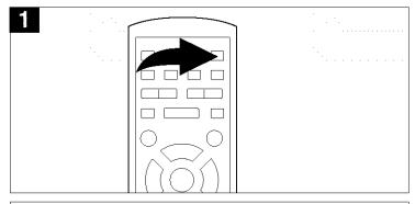
Press the STANDBY ON/OFF button on the main unit/remote to turn on the unit; the STANDBY indicator will go out and the Backlights will turn on.
