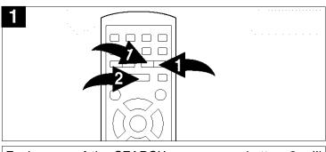
Each press of the SEARCH ►► or ◄◄ button ● will increase the search as follows: 1st press: x 2 2nd press: x 4 3rd press: x 8 4th press: x 20 5th press: Resume Normal Playback Press the PLAY (►) button ❷ to resume normal playback. REPEAT PLAY
