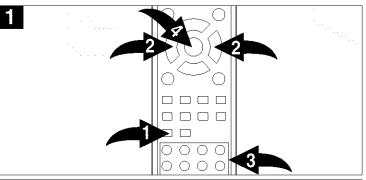
Press the SEARCH button **①**. Press the Navigation  $(\blacktriangleleft, \triangleright)$  buttons **②** to select the TIME, then use the Number buttons **③** to select the desired time (Hour/Minutes/Seconds). Press the ENTER **④** button and playback will start immediately.
