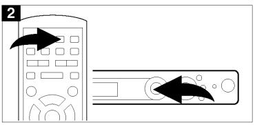
Press the OPEN/CLOSE button to open the disc tray, "OPEN" will appear on the screen and in the display. Insert an MP3 disc with the label side facing up on the disc tray.
