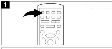
Press the MUTE button once to mute the sound, "MUTE" will appear on the TV screen. Press the MUTE button again to restore the sound; "DEMUTE" will appear on the TV screen for three seconds.
