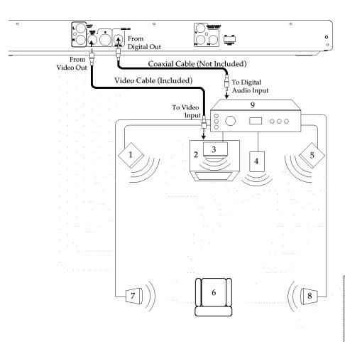
Place the subwoofer, front, rear and center speakers in locations as shown/described here. After correctly positioning the speakers, perform the Tone Test on the AV Amplifier and adjust the volume controls until the desired sound is achieved. For best results, sit in the viewing position and have someone adjust the volumes for you; this will enable you to set the optimal levels.
