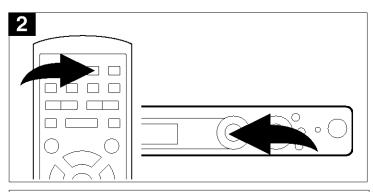
Press the OPEN/CLOSE button to open the disc tray, "OPEN" will appear on the screen and in the display. Insert a disc will the label side facing up on the disc tray.
