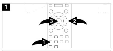
During playback of a disc, press the 3D button ● once and the sound options will appear on the screen. Press the ► button ④ to select SRND, then press the (▲, ▼) buttons ④ to select a surround mode (OFF, CONCERT, CHURCH, PASSIVE, WIDE or LIVE). Press the ENTER button ❸ to confirm. Press the 3D button ❶ to exit.
