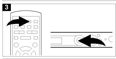
Press the OPEN/CLOSE button to close the disc tray. "LOAD" will appear on the screen and in the display. After loading, playback will start automatically.
