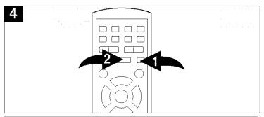
To stop playback, press the Stop ( $\blacksquare$ ) button  $\bullet$ ; "PRESS PLAY TO CONTINUE" will appear on the TV screen. Because the unit will remember where you stopped, simply press the Play ( $\triangleright$ ) button  $\bullet$  to resume playback where you left off (resuming playback). If the Stop ( $\blacksquare$ ) button  $\bullet$  is pressed twice, the unit will stop completely.
