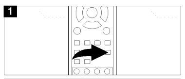
Press the AUDIO MODE button to cycle through the audio modes. The audio modes vary depending on the disc inserted, but include MONO LEFT, MONO RIGHT, STEREO.
