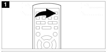
Press the STANDBY ON/OFF button on the main unit/remote to turn on the unit; the STANDBY indicator will go out.
