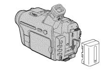
With the ▲ mark on the DC plug facing up, connect the AC Adaptor to the DC IN jack on your camcorder.
