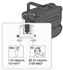
\* The minimum distance required between your camcorder and the subject to get a sharp focus in that position of the lever. Move the power zoom lever slightly for a slower zoom. Move it further for a faster zoom.
