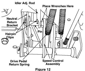
• Remove both hairpin clips from the pin which is fastened to the speed control assembly (be careful not to lose the small flat washers on the pin). See Figure 12.
