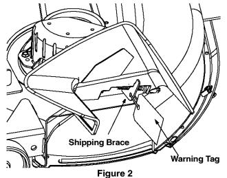
While holding the discharge chute with your left hand, remove the shipping brace with your right hand by grasping it between your thumb and index finger and rotating it clockwise.
