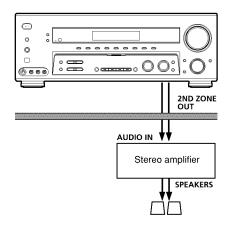
Press 2ND ZONE repeatedly to select the analog audio signals for output to a stereo amplifier in another room. For details on the connection, see page 15.
