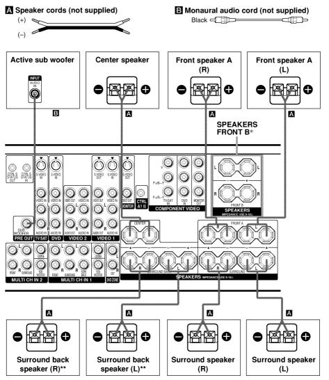
\* If you have an additional front speaker system, connect them to the SPEAKERS FRONT B terminals. You can select the front speakers you want to use with the SPEAKERS (OFF/A/B/A+B) button (page 26).
