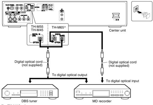
Before connecting a digital optical cord, unplug the protective plug.
