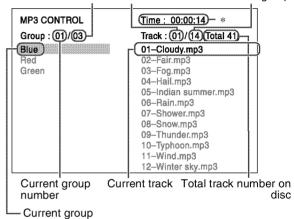
\* Elapsed playing time of current track Elapsed playing time is only shown during playback.
