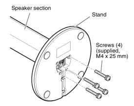
Repeat the procedure from step 1 to assemble the other satellite speakers.
