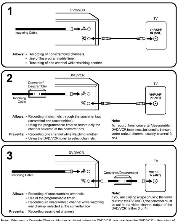
Note: Whenever a Converter/Descrambler box is placed before the DVD/VCR, you must tune the DVD/VCR to the output of the Converter/Descrambler box, usually channel 3 or 4.
