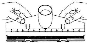
3. Press down with each thumb below the latching tabs until you see and hear the removable insert snap into the nozzle body. Snap the latches over the locking tabs into their original position.
