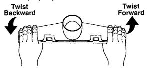
The wet nozzle assembly is ready for wet pickup use.
