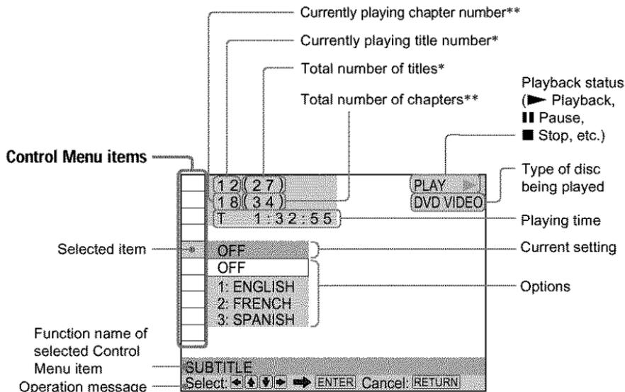
\* Displays the scene number for VIDEO CDs (PBC is on), track number for VIDEO CDs/ Super audio CDs/CDs, album number for DATA CDs.
