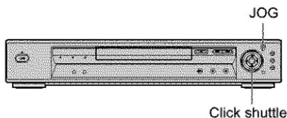
Turn the click shuttle on the player. The playback speed changes depending on the turning direction and degree of rotation as follows:
