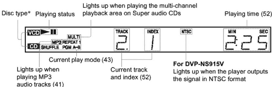
\* When playing the HD layer of Super Audio CD discs, the disc type is not displayed.
