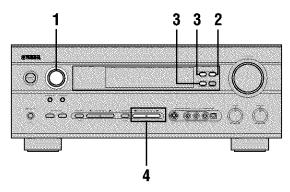
1 **Rotate the INPUT selector (or press TUNER** on the remote control) to select TUNER as the input source.
