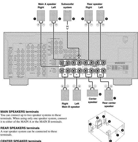
A center speaker can be connected to these terminals.
