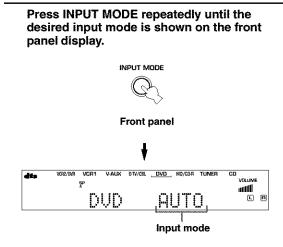
AUTO: In this mode, the input signal is selected automatically as follows:
