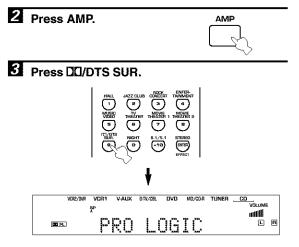
The display cycles as follows each time you press DD/ DTS SUR :
