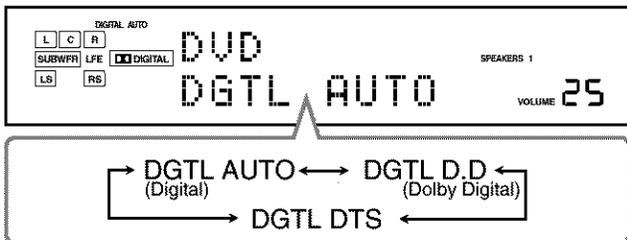
When “DGTL D.D” or “DGTL DTS” is selected, the AUTO indicator goes off, and the corresponding digital signal format indicator lights up on the display.
