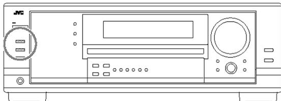
To use the speakers connected to the **FRONT SPEAKERS ① terminals**, press **SPEAKERS ON/OFF 1** so that the **SPEAKERS 1** indicator lights up on the display. Make sure that the **SPEAKERS 2** indicator is not lit on the display.
