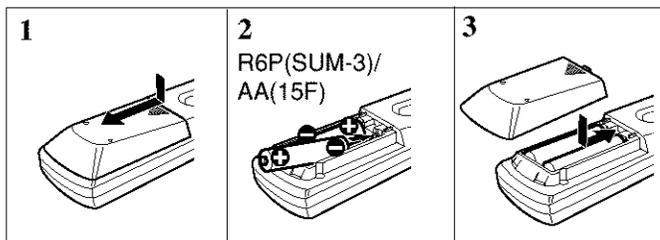
1. Press and slide the battery cover on the back of the remote control.
