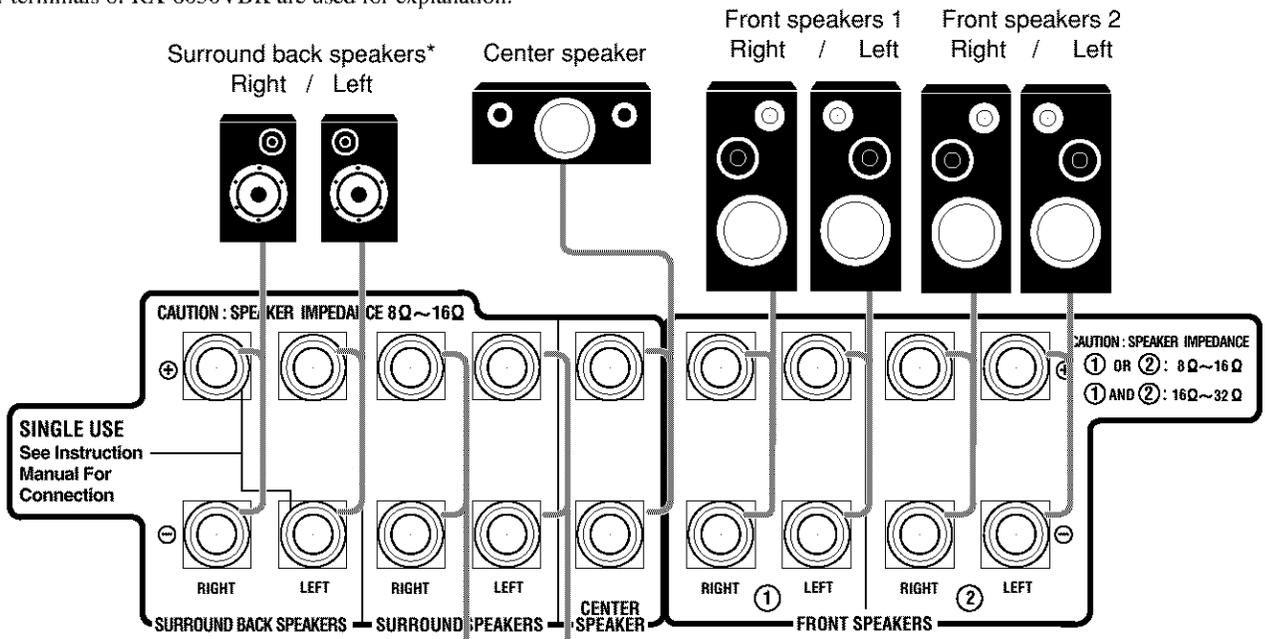
\* When using only one surround back speaker, connect the ⊕ cord to the RIGHT ⊕ terminal and the ⊖ cord to the LEFT ⊖ terminal.
