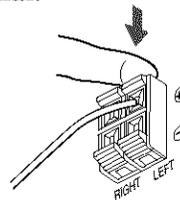
For each speaker (except for a subwoofer), connect the (+) and (-) terminals on the rear panel to the (+) and (-) terminals marked on the speakers.
