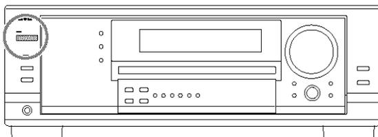
Press **STANDBY/ON** (or **AUDIO** **STANDBY/ON** on the remote control).
