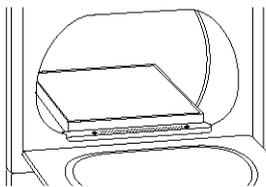
3. Place wet items on top of the rack. Allow space around items for air to circulate. The rack does not move, but the drum will rotate. Make sure items do not hang over the edges or between rack grill.
