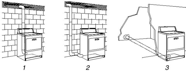
1. Standard rear offset exhaust installation
