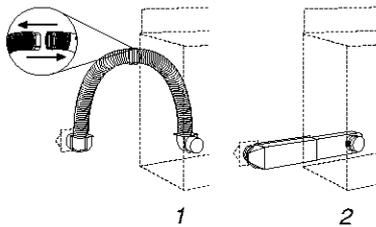
1. Over-The-Top installation (also available with one offset elbow)
