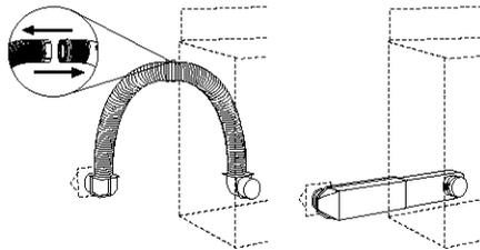
1. Over-The-Top installation (also available with one offset elbow)
