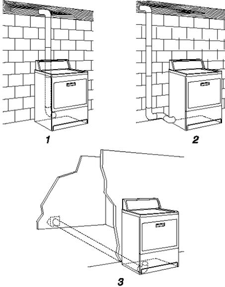
1. Standard rear offset exhaust installation
