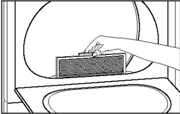
**STEP 2.** Roll lint off the screen with your fingers. Do not rinse or wash screen to remove lint. Wet lint is hard to remove.
