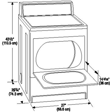
**Recommended installation spacing for recessed area or closet installation**
