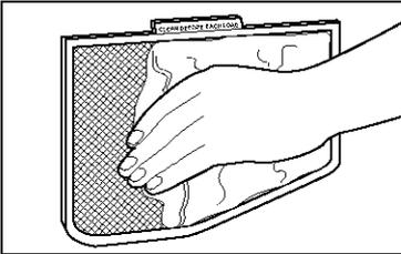
**STEP 3.** Push the lint screen firmly back into place.
