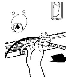
3. Cut the shipping strap about 16 in. (41 cm) from plug end. Look for the words "CUT HERE." Discard end with the cotter pins. Slide remainder of shipping strap from the power cord.
