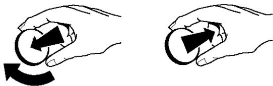
Pull out the Cycle Selector Control (Timer) knob to start the washer.
