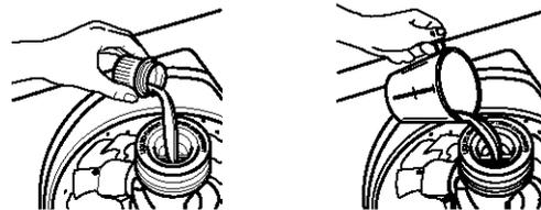
Dilute liquid fabric softener by filling the dispenser with warm water until liquid reaches the bottom of the opening of the funnel-shaped portion of the dispenser.
