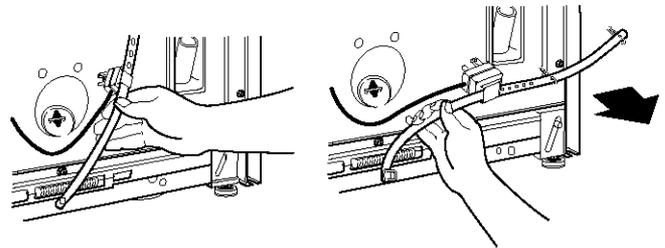
2. Pull firmly to remove the end of the shipping strap that remains pinned to the back of the washer. This will release the rear self-leveling feet.
