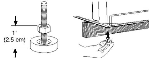
3. Screw the feet into the correct holes at the front corner of the washer until the nuts touch the washer.
