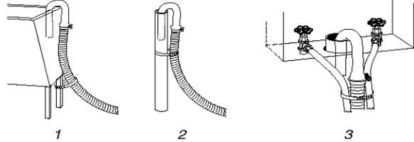
If the washer faucets and the drain standpipe are recessed, put the hooked end of the drain hose in the standpipe. Tightly wrap the tie strap around the water inlet hoses and the drain hose. (See illustration 3.)
