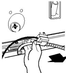
3. Cut the shipping strap about 16 in. (40 cm) from plug end. Look for the words "CUT HERE." Discard end with the cotter pins. **Slide remainder of shipping strap from the power cord.** You will use the remainder of the shipping strap later to secure the drain hose.
