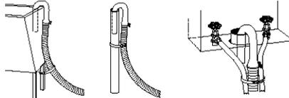
If the washer faucets and the drain standpipe are recessed, put the hooked end of the drain hose in the standpipe. Tightly wrap the tie strap around the water inlet hoses and the drain hose.
