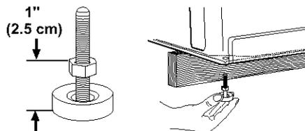
3. Screw the feet into the correct holes at the front corner of the washer until the nuts touch the washer.
