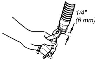
4. Open clamp. Twist hose back and forth while pushing down onto drain connector at the bottom of the washer. Continue until hose contacts the ribbed stop on the cabinet.
