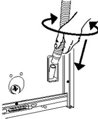
5. Place clamp over area marked "CLAMP." Release clamp.
