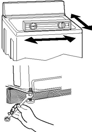
If the washer is not level, move the washer out slightly, tip back, prop up the front of the washer with the wood block and adjust the feet up or down as necessary. Repeat this step until washer is level.
