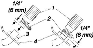
**For standpipe or laundry tub drain systems:**
