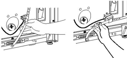
2. Pull firmly to remove the end of the shipping strap that remains pinned to the back of the washer. This will release the rear self-leveling feet.
