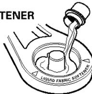
Dilutes fabric softener and adds it to the rinse at the correct time to prevent softener staining.
