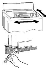
If the washer is not level, move the washer out slightly, tip back, prop up the front of the washer with the wood block and adjust the feet up or down as necessary. Repeat this step until washer is level.
