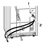
1. Cold water inlet valve (blue) 2. Hot water inlet valve (red) **NOTE:** The inlet valve may be on the right or the left side of the washer, depending on your model.
