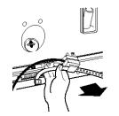
Cut the shipping strap about 16 in. (40 cm) from plug end. Look for the words "CUT HERE." Discard end with the cotter pins. Slide remainder of shipping strap from the power cord. You will use the remainder of the shipping strap later to secure the drain hose.
