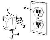
1. 3 prong grounding plug 2. 3 prong grounding-type outlet 3. Ground prong 4. Power supply cord
