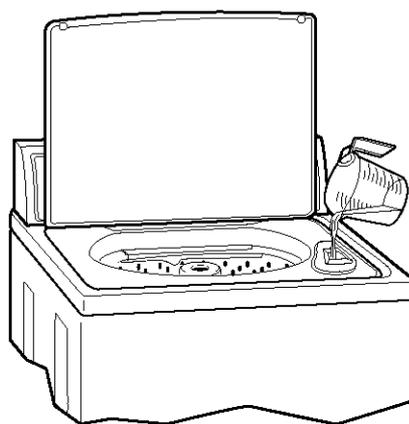
After loading the washer, pour measured liquid chlorine bleach carefully into the dispenser.
