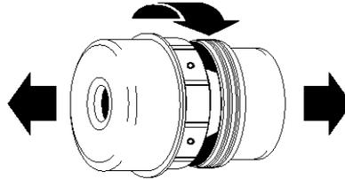
**STEP 3.** Remove internal holding cup.
