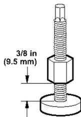
**STEP 3.** Screw leg into washer base by hand until nut reaches washer base. Repeat for other leg.
