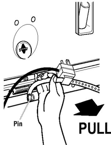
**STEP 3.** Cut the shipping strap about 16 inches (40 cm) from plug end. Look for the words "CUT HERE." Discard end with the cotter pins. **Slide remainder of shipping strap free from the electrical plug.** You will use this to secure the drain hose.
