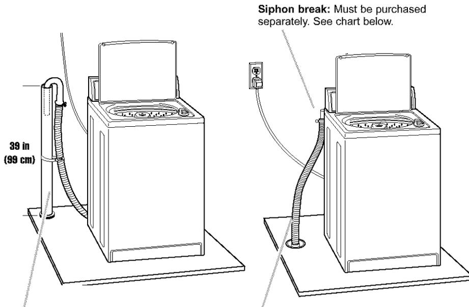
**Standpipe drain system:** Needs a 2 in (5 cm) minimum diameter standpipe with minimum carry-away capacity of 17 gal (64 L) per minute. Top of standpipe must be at least 39 in (99 cm) inches above floor and no higher than 96 in (2.4 m) from bottom of washer.
