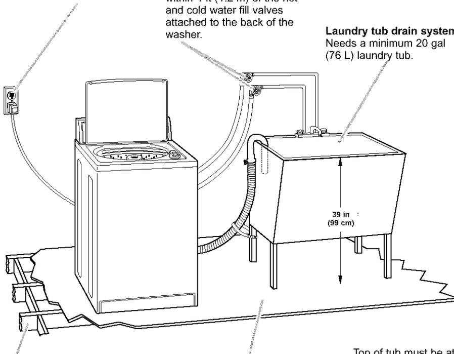
**Support:** Floor must be sturdy enough to support a total weight of 315 lbs (143 kg) (including washer, water, and load weight).
