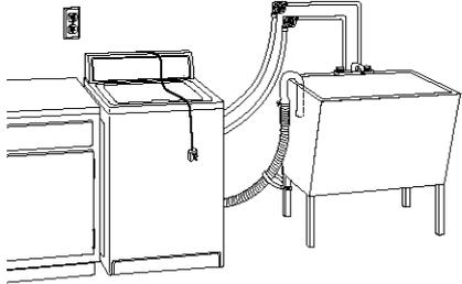
**STEP 2.** Locate the remaining piece of shipping strap (not the end with the cotter pins) from STEP 3 of "REMOVE SHIPPING STRAP." Use it to wrap the drain hose together with the laundry tub or standpipe. Push fastener into the nearest hole in the shipping strap.
