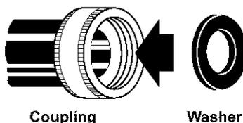
**STEP 2.** Attach the hose with the red coupling to the hot water (bottom) inlet valve. Attaching the red coupling first makes it easier to tighten connection with pliers. Screw on coupling by hand. Make an additional two-thirds turn with pliers to tighten coupling. **DO NOT OVERTIGHTEN;** this could damage the valves.
