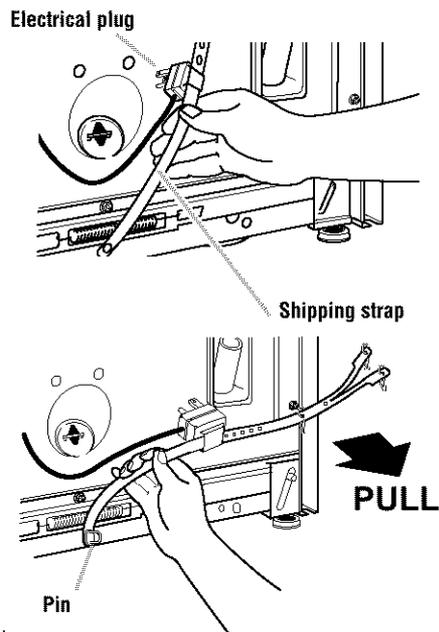
**STEP 2.** Pull firmly to remove the other end of the shipping strap pinned to the back of washer. This will release the rear self-leveling legs.
