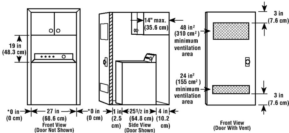
\*Additional clearance for wall, door and floor moldings may be required.
