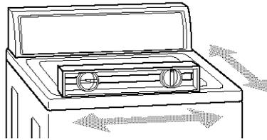
**STEP 7.** If washer is not level, prop up the front of the washer and adjust the legs up or down as necessary. Lower washer and reset self-adjusting rear legs (as in Step 6). Repeat Step 7 until the washer is level.
