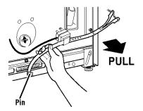
**STEP 2.** Pull firmly to remove the other end of the shipping strap pinned to the back of washer. This will release the rear self-leveling legs.
