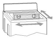
STEP 7. If washer is not level, prop up the front of the washer and adjust the legs up or down as necessary. Lower washer and reset self-adjusting rear legs (as in Step 6). Repeat Step 7 until the washer is level.
