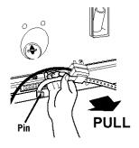
STEP 3. Cut the shipping strap about 16 in (40 cm) from plug end. Look for the words "CUT HERE." Discard end with the cotter pins. Slide remainder of shipping strap free from the electrical plug. You will use this to secure the drain hose.
