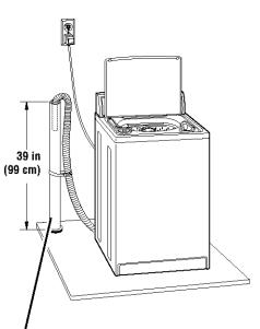
Floor drain system: Requires a siphon break, see chart below. A minimum carry-away capacity of 17 gal (64 L) per minute is required.
