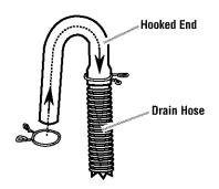
**STEP 3.** Put hooked end of drain hose into laundry tub or standpipe. Check for proper length of drain hose. Rotate hook to eliminate kinks.
