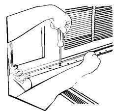
**C** Extend the left and right accordion panels to the vertical window sashes, drill 1/8" pilot holes, and attach the top corners with 2 Type B screws. Use an accordion panel clamp on each lower corner to trap the panels. Drill 1/8" pilot holes and attach the panel clamps with Type B screws.
