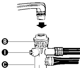
Turn water faucet off. Press bleeder button **I** on hose connector **C** to release water pressure. Pull down on locking collar **B** and hold while removing hose connector from faucet. Turn hose connector upside down and empty water from inside connector.
