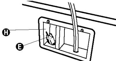
Unplug power supply cord **E** and insert cord into storage compartment **H**.
