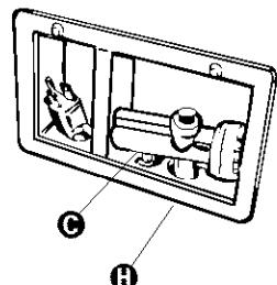
Insert inlet/drain hoses and hose connector **C** into storage compartment **H**.
