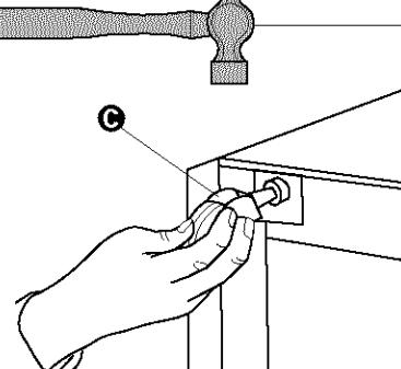
Insert casters **C** into holes at corners of dishwasher. Lightly tap casters with a small hammer until they lock in place.
