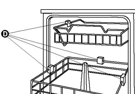
Stand dishwasher upright. Open door and remove beaded foam shipping pieces **D** from racks. Close dishwasher door. Latch dishwasher door shut.
