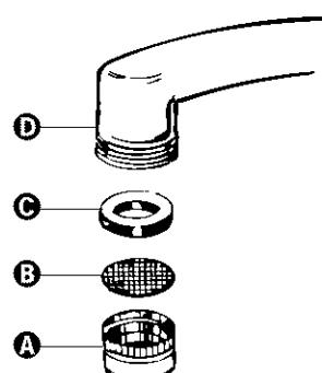
Remove screen holder or aerator **A**, screen **B** and washer **C**, from end of faucet **D**.
