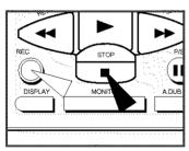
Press REC for at least one second to start recording. When you have finished recording, press STOP (■).
