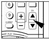
Insert the cassette. Select the channel by pressing the CH buttons ( $\blacktriangle$  or  $\blacktriangledown$ ) on the remote control.
