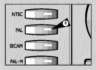
You can convert the signal recorded on a tape to another format on a second tape.
