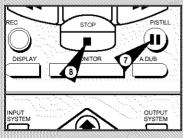
This function enables you to start a new recording at a specific position on the cassette while maintaining a very smooth scene change.
