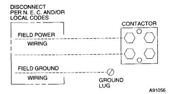
Fig. 4—Line Power Connections
