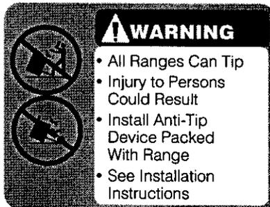
These **ANTI-TIP** bracket installation instructions are for wood or concrete floors and walls. Any other type of construction may require special installation techniques to provide adequate fastening of the **ANTI-TIP** bracket to the floor and wall.
