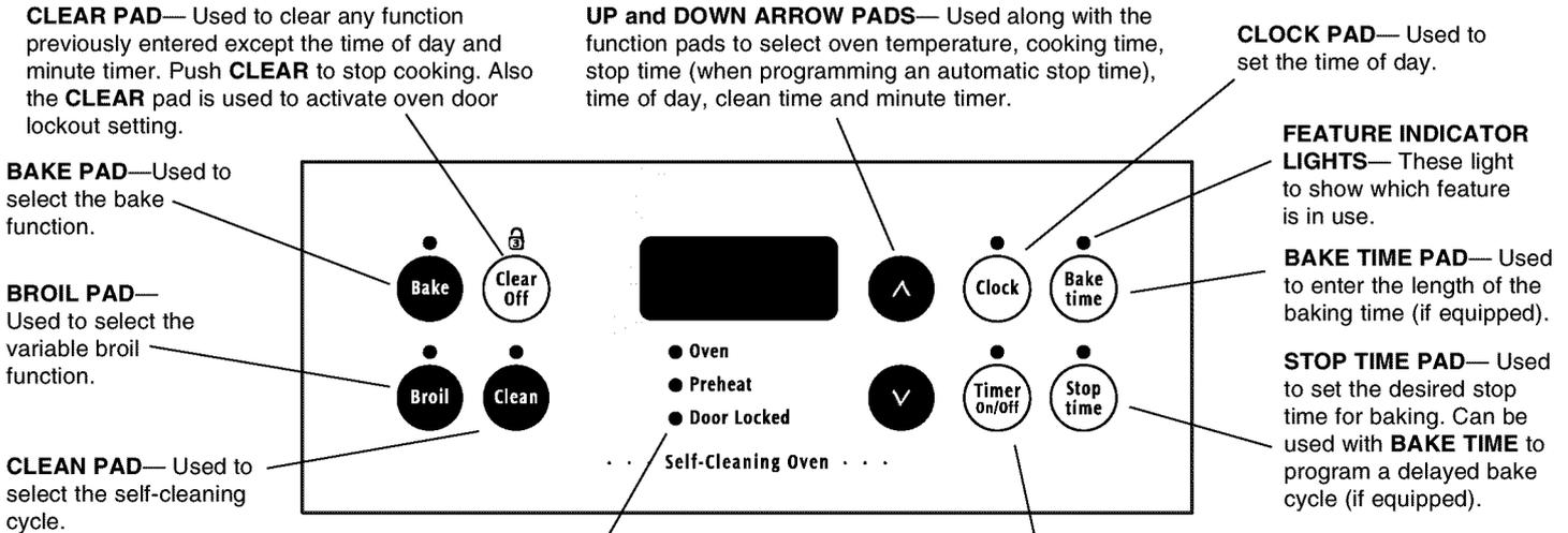
**The oven can be programmed to: BAKE, TIME BAKE, BROIL, SELF-CLEAN, CONTINUOUS BAKE and set for OVEN LOCKOUT.**
