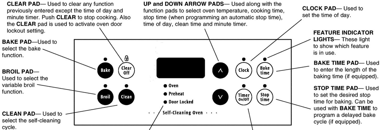
**OVEN, PREHEAT & LOCK LIGHTS**— The "OVEN" light will glow each time the oven turns on to maintain the set oven temperature. The "PREHEAT" light will glow when the oven is first set to operate, or if the desired temperature is reset higher than the actual oven temperature. The "DOOR LOCKED" light will flash when the oven door locks and unlocks or when using the self-clean cycle or the oven door lockout mode is activated. The indicator light will glow constantly after the door locks.
