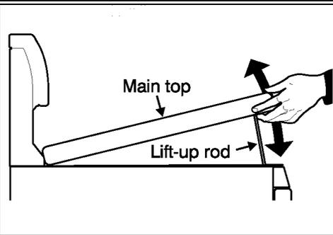
**CAUTION** When lowering the lift-up range top, grasp the sides with fingertips only. Be careful not to pinch fingers. **DO NOT** drop or bend the range top when raising or lowering. This could damage the surface.
