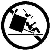
**⚠ WARNING** To reduce the risk of tipping, the range must be secured by properly installed anti-tip bracket provided with the range. To check if the bracket is installed properly, visually check that rear leveling leg is inserted into and fully secured by the anti-tip bracket by removing lower panel or storage drawer. Refer to the Installation Instructions for proper anti-tip bracket installation.
