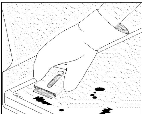
If soils remain, carefully scrape soils with a metal razor blade scraper, holding scraper at a 30 degree angle to the surface. Remove loosened soils with cooktop cleaning cream and buff surface clean.
