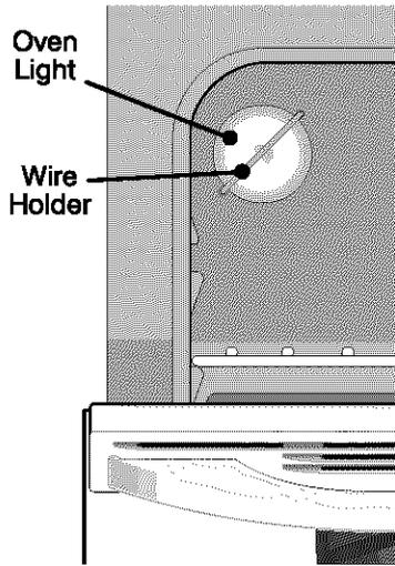
On some models, the oven light automatically turns on when the door is opened. Some models have a switch located on the control panel to turn on the light. The oven light is located at the rear of the oven and is covered with a glass shield held by a wire holder. The glass shield must be in place whenever the oven is in use.
