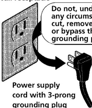
Power supply cord with 3-prong grounding plug
