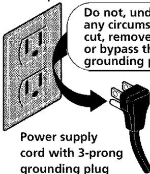
Power supply cord with 3-prong grounding plug
