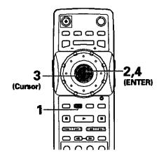
Move the cursor control joystick to select one of the preprogrammed picture quality settings. Standard\*: Preset that presents the source video as it is, with no special adjustments.
