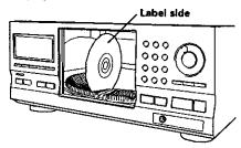
4 Press SELECT DISC NUMBER (the dial mode indicator lights green) and then turn MULTI DIAL to rotate the rack to the next position.
