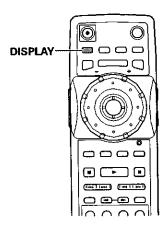
Press **DISPLAY** during while a disc is playing. Press **DISPLAY** repeatedly to change the information being displayed.
