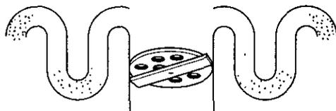
9. Fresh, hot water enters the dishwasher and sprays on the dishes. The rinse water is then pumped through the ULTRA WASH soil removal system and remaining soil is removed.
